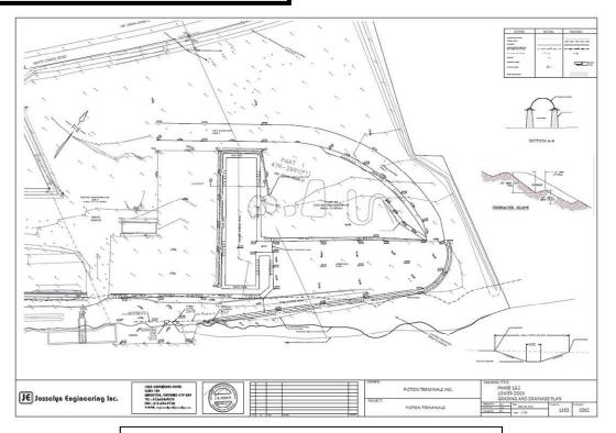
Drawing of proposed interim stormwater plan during construction of Dry Storage for bulk materials like road salt. Drawing by Josselyn Engineering
